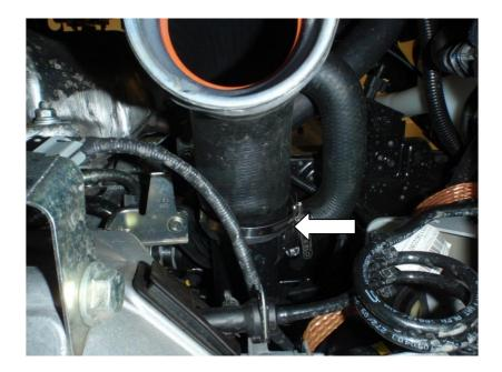
13. From under the car looking up again you will see the rubber hose you have just disconnected from the metal pipe, again the 'use once' clip must be broken and then remove rubber hose.
