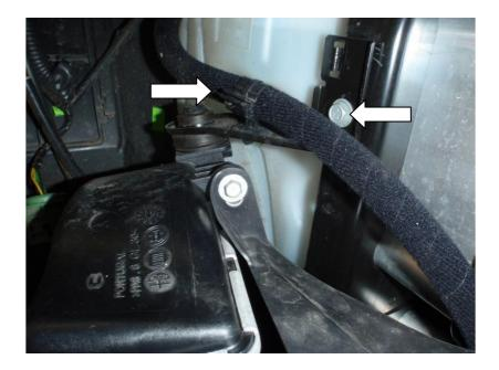
**15.**Undo the clip holding the washer bottle pipe and undo the 10mm bolt on the driver's side, you will now be able to remove the complete intercooler unit by pulling upwards with an even force to release the bottom pegs from the rubber grommets.
