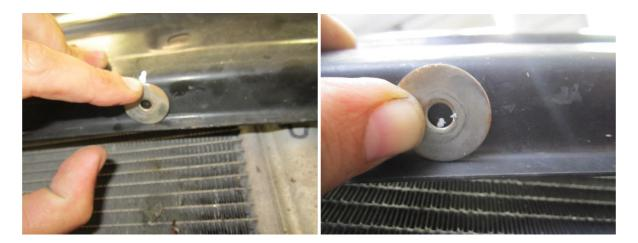
**22.** Drill two holes with a pilot drill as pictured below then enlarge the holes to 9mm with a larger drill bit.
