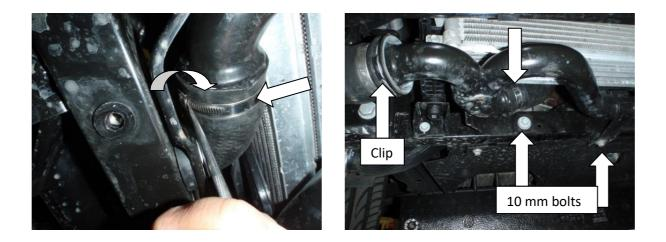
8. Now the bumper is off you will see a large black pipe which is connected to a rubber hose from the turbo, it has a 'use once' only clip this must be broken to remove. Undo the two 10mm bolts holding the pipe to the chassis and pull the clip out which is holding the hose to the pipe.
