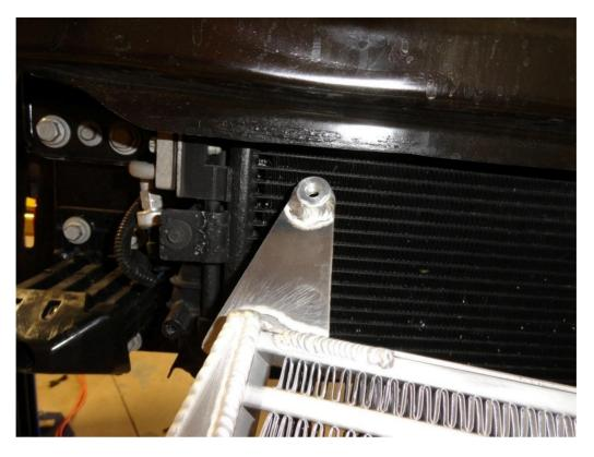
**18.** FOR U.S. CUSTOMERS AND VEHICLES SUPPLIED WITHOUT A LOWER CRASH BAR: Push the mounting tabs on the intercooler up behind the crash bar so that the bosses on the ends line up with the holes already in the crash bar.
