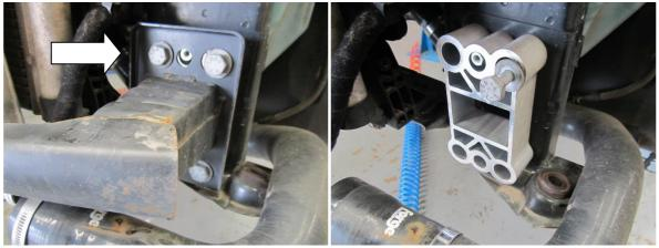
**20.** Hold your new forge motorsport intercooler up to the center of the middle crash bar and mark the boss locations with a paint marker.
