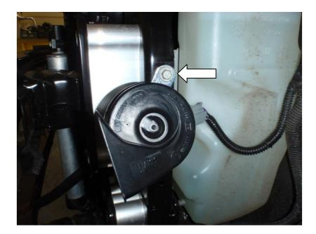
**17.** Using the bolt that was holding the intercooler move the horn up to the existing threaded hole and replace the bolt relocating the horn in a new position.
