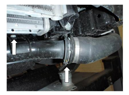
9. At the other end of the pipe, undo the last 10mm bolt, which secures the pipe to the chassis, using the 10mm ratchet spanner, and pull the clip out which is holding the hose to the pipe. This pipe is now free and can be taken off the car.
