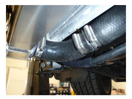
**27**. Push the long silicon hose onto the intercooler with a 55mm jubilee clip and do up in such a way that the bulky part of the clip is not on the bottom of the pipe because the intercooler sits slightly lower than stock. Place the 45mm hose joiner supplied in the open end of the hose and secure with a jubilee clip.
