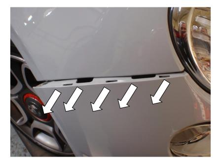
**6.** Pull the bumper away from the wing in the direction of the arrows with a firm but even pressure, taking care not to bend the bumper too much as this may crack the top edge.
