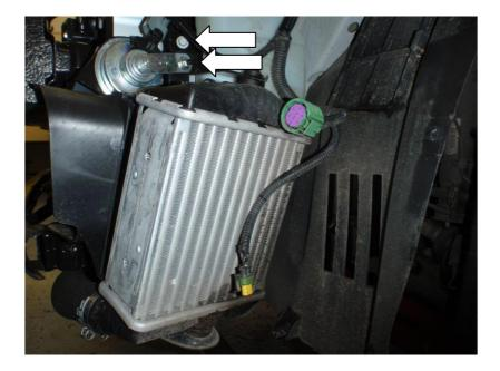
**16.**Undo the 10mm bolt and the 10mm nut holding the horn and intercooler on the passenger side, you will now be able to remove the complete intercooler unit by pulling upwards, with an even force to release the bottom pegs from the rubber grommets.
